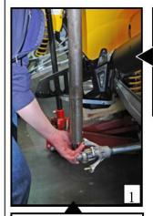
To remove the castle nut move the wrench counter clockwise.
