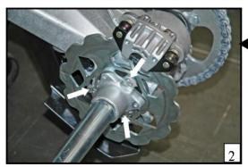
Remove the 3 bolts that hold the bolt keeper, brake hub and secures the axle retaining ring on. You may have to bend the tabs back to get the socket around the bolts.
